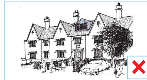
Fig B.54 Avoid bulky dormers unsympathetic to the building elevation.
