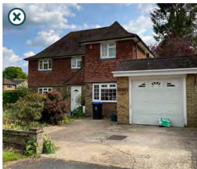
Figure 48: Negative example of on-plot parking with attached garage at the side of the building, dominating the principle building line, with impermeable driveway ground surfacing.
