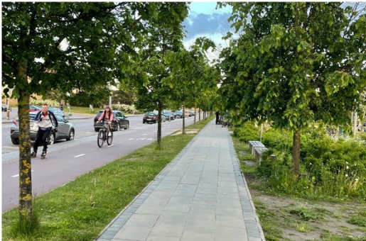
Walking and cycling routes with trees and green verges separated from vehicular movement by parked cars
